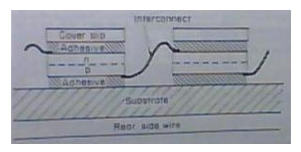
In essence, the usage of solar power systems onboard satellites uses photovoltaic systems. Photovoltaic system is when the production of power across the junction of two dissimilar materials (n and p doped semiconductors) take place when exposed to light or electromagnetic radiation.
